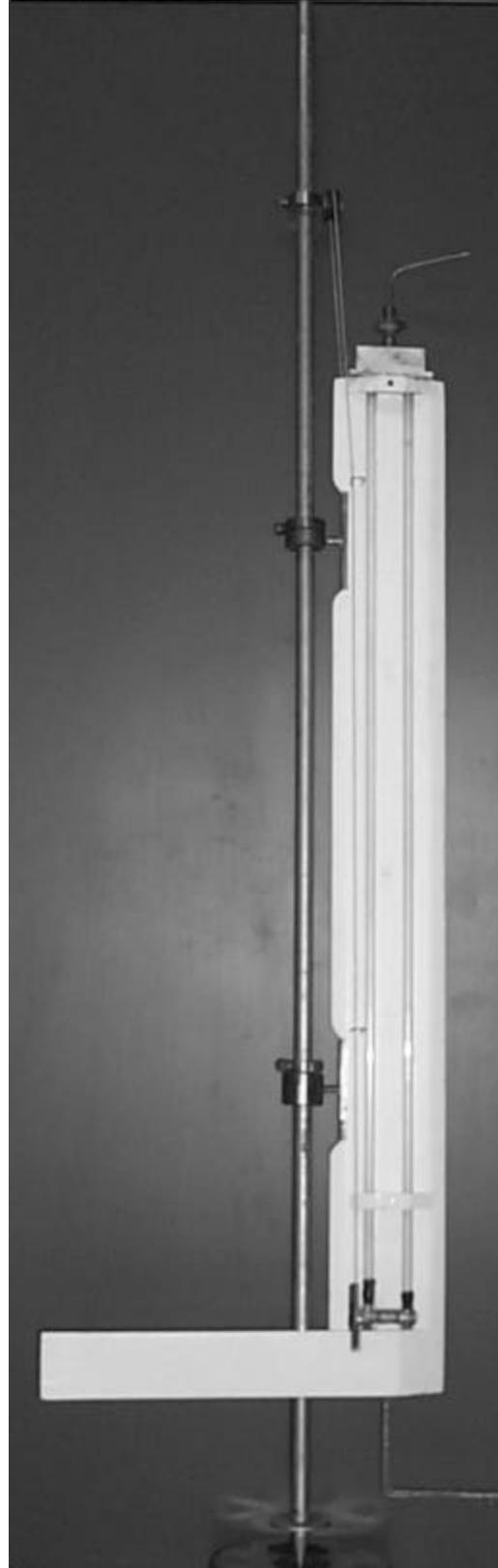
Figure 5. Replica of 1856 Pitot-Darcy tube.
