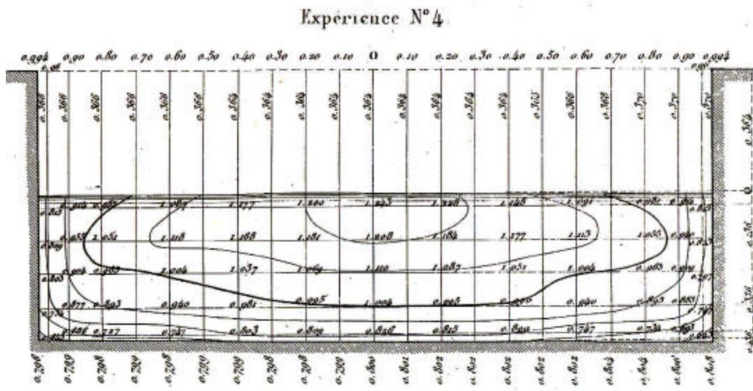
Figure 8. Example of open channel isovels from Darcy and Bazin (1865).
