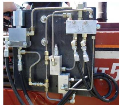
**Figure 16: Hard Lined Valve Plate**
