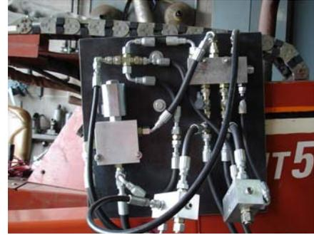
**Figure 23: Mounted Valve Plate**
