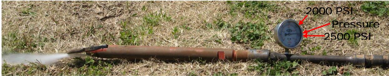
**Figure 30: Full Drill String Pressure Reading**
