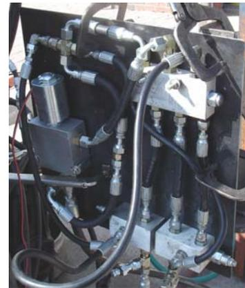
**Figure 15: Valve Plate**
